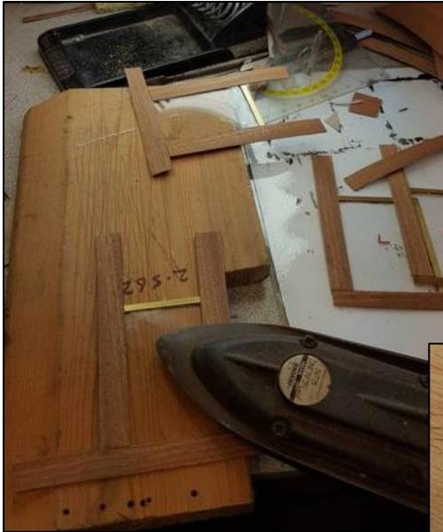
Here we have the other edge covered and also showing the tool used for ironing the veneer on. This iron is over 20 years old, from my days of R/C aircraft, this iron was used for covering wooden frames in 'Solartex or solarfilm' and was perfect for this particular job, I set the temp for 300c.
