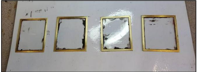
Once the window frames and glass had been cleaned, I sanded down the brass frame for a better bond, preparing them so that the long process of covering the outside edges with a wooden veneer could begin.
