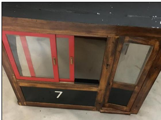
With the cab now complete it was removed and the wood treated with a wood stain. The steel panels in the doors and the roof will be painted when the repairs to the rest of the engine have been completed. The whole assemble together with the unpainted bunker was carefully put to one side ready for final assembly.
