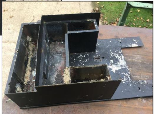
So, it was removed from the frames, taken apart and the various bits cleaned up. Then the whole assembly was reassembled and soldered up to give a fully watertight tank. Repainting will follow.
