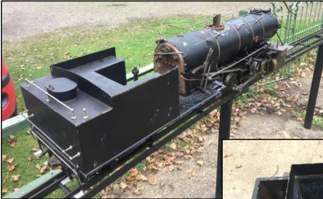
With the valve gear and cylinders refurbished attention now turned towards the cab and bunker. The tank had been sealed previously with a mix of filler and other sealants.
