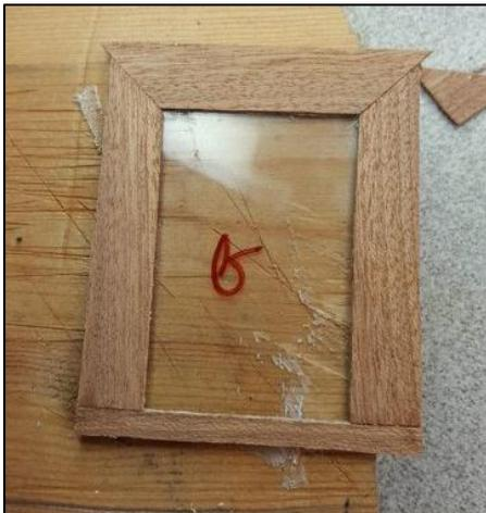
frame is made with square joints at the bottom (mortise and Tenon perhaps) and angled cuts for the tops. In the next picture you can see where the sides butt up against the bottom and the 45-degree cuts that I have cut for the top. What I am doing here is keeping the grain direction as per prototype.
