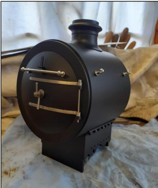
Next up was the fitting of the smokebox door ring to the smokebox barrel. Now to ensure that the smokebox door hinges are parallel with the frames I used a digital angle gauge which I set to zero on the saddle frame and then offered it up to the smokebox door hinge brackets and keeping the zero setting from the frame as the door ring was tapped home, note that I added a thin film of silicon sealant to the door ring prior to fitting to aid an airtight seal.
